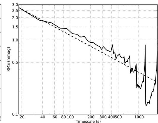
Fig. 5: Precision varies with binning of data in 16 Cygnus A light curve. Once binned down to timescale of ~200s (or 3 min), the observational scatter of newly binned light curve is proven to be  $< 1$  mmag [2].
