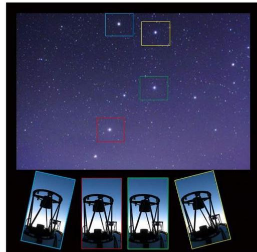
Fig. 2: Demonstration of MINERVA's 4 telescopes observing distinct regions of the sky (Credit: Miguel Claro). Figure 1 showed how one telescope's field of view usually contains very few—if any—bright stars. With MINERVA, 3 additional telescopes are used to find those necessary comparison stars that are as bright as our primary star with the transiting exoplanet(s).
